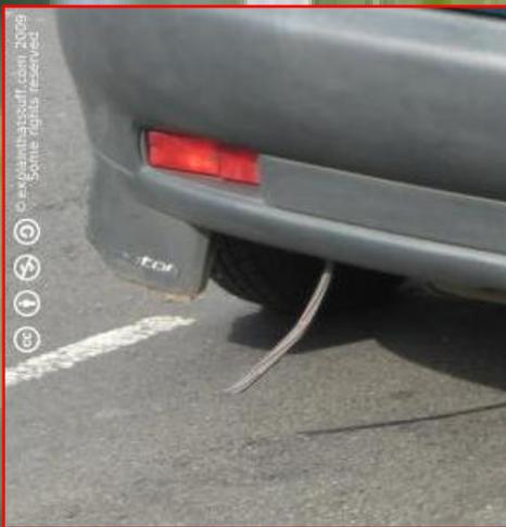
Photo (left): An anti-static car strip. Look closely and you'll see a zig-zag of copper wire running across the surface. This is what carries the static electricity to the ground.
